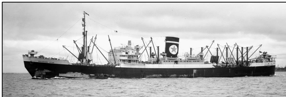
Brisbane Star (11,124/1937) arriving Melbourne 14 February 1946, still with temporary bow, Carley floats, 4" guns fore and aft and six A/A gun emplacements in situ . (A.C.Green/State Library of Victoria)
